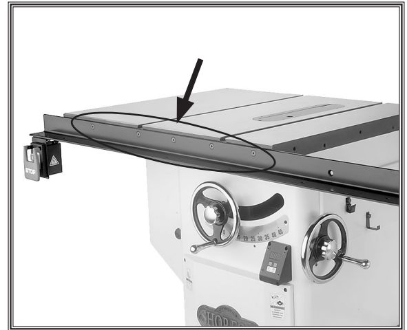
Figure 13. Front rail installed.
